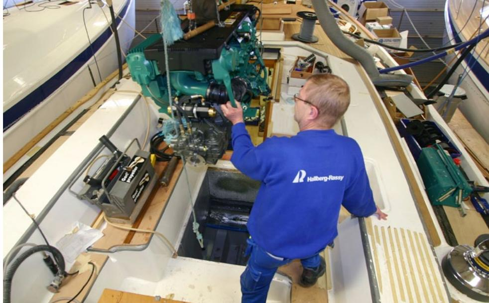
*Engine and tanks come in through the normal opening of the boat after that the woodwork is done*
