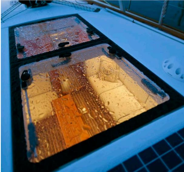
*Flush mounted deck hatches*
