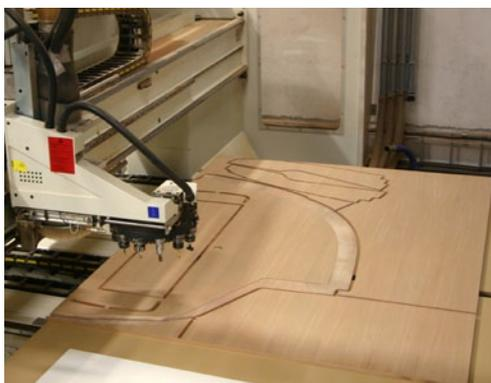
*Computerised controlled machines for cutting
