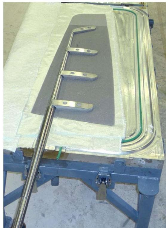
*The rigid rudder has a solid stainless shaft (no pipe) that is moulded into the solid rudder blade*
