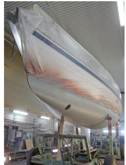
*Two coats of epoxy primer and two coats of antifouling applied as standard*
